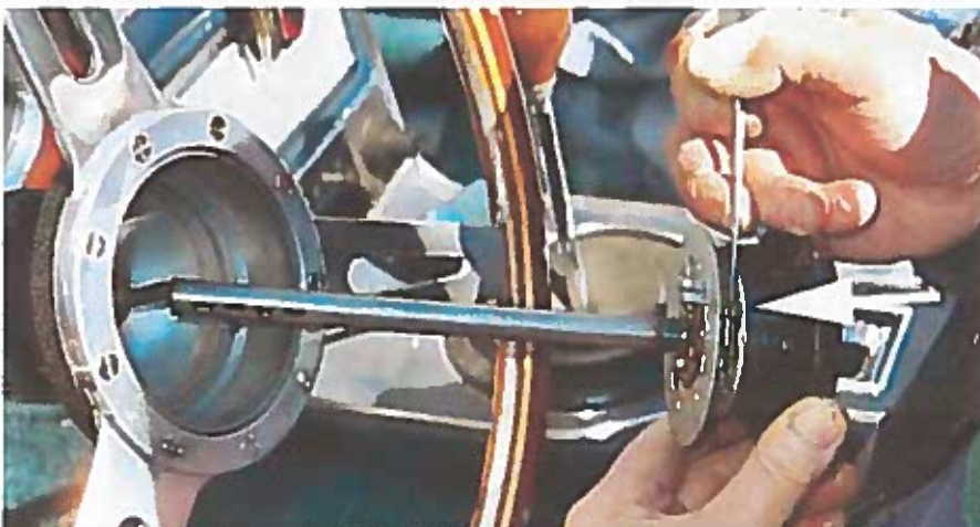
Photo 13: With the sliding stator pulled out several inches, you have easy access for removing the switch.
