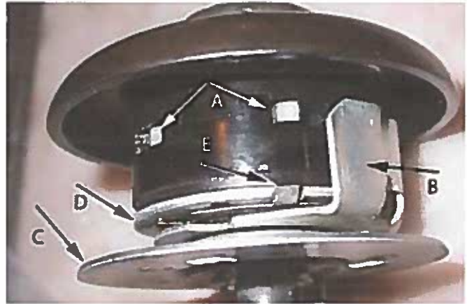
Photo 9: This wavy steel cancelling design was used on later 100s with adjustable steering up to BN1 C.149929 when non-adjustable columns were introduced. The pawls (A) (common to ALL turn signal switches) were tripped by a heavy steel wavy plate (B) that is connected to the moving plate (C). The fixed plate (D) mounts to the Bakelite switch with three screws, as with all switch configurations. The tab (E) positions a thin cover plate to keep the mounting screws from falling out.
