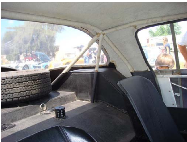
Interior exhibits the small diameter tubing which made up the frame of the race car—no large roll cage here!
