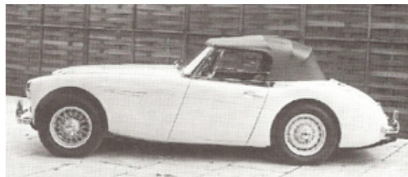
The Austin-Healey 3000 MK II, Series BJ7, showing wind-up side windows and a true convertible top. Its interior retained the style of the previous models.
