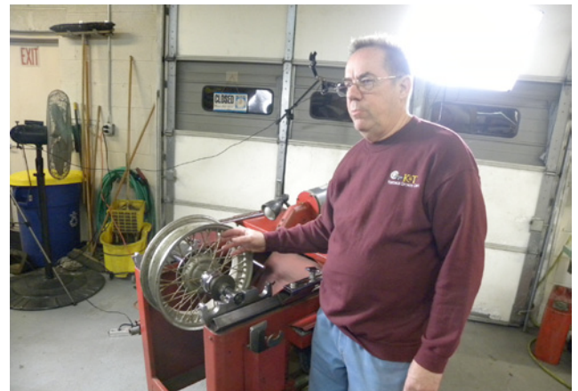
Ken Beck demonstrates wire wheel truing at LV
