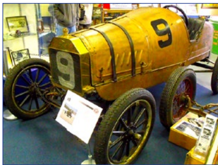
Early Model-T racer. This beast had no gear box and no brakes, "to save weight."
