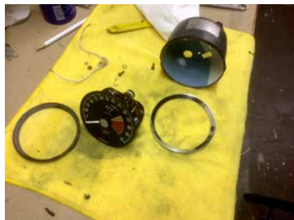
Tach disassembled showing case, bezel and glass Tach disassembled showing case, bezel and glass.
