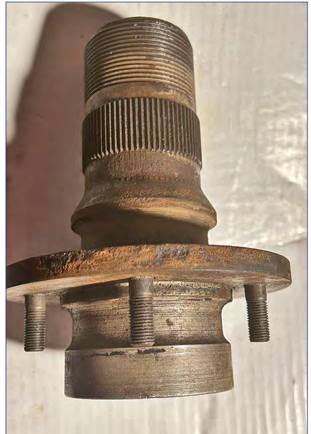
Right front wheel hub with its brake disk removed.
