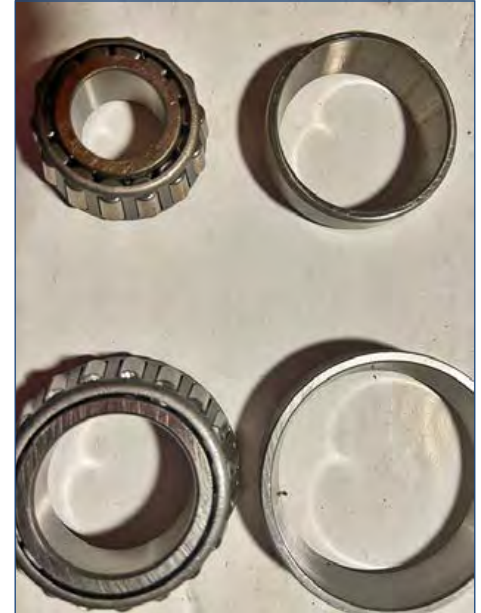
Small outer bearing and its race are shown on top, with a larger inner bearing and its race shown beneath.
