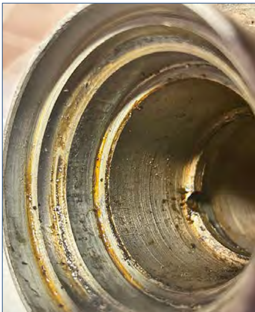
Close-up view of the inner hub showing the small slot on the inside ridge.
