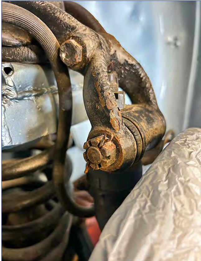
3 Only two bolts need to be removed to replace the top kingpin bushings.
