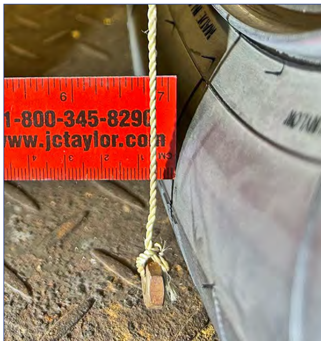
8 Driver side camber was the worst, 7mm outward tilt before bushings installed.
