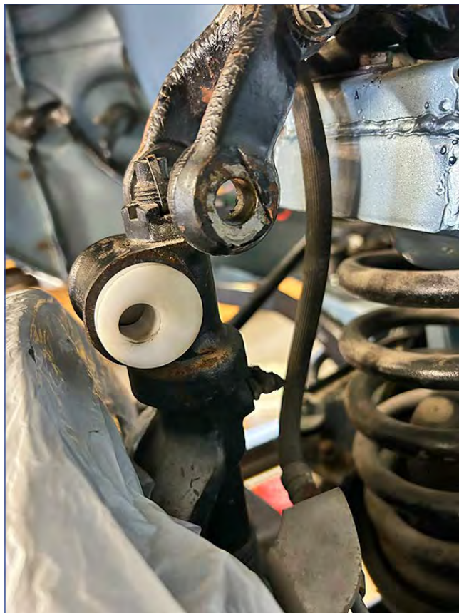
6 New eccentric bushings in place. Note they are currently installed to move the top of the wheel outward. I rotated them toward the center of the car to bring the top of the wheel inward.
