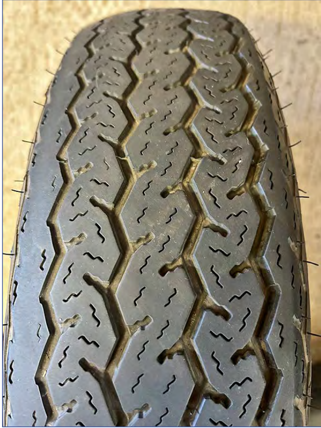
1 Noticeable wear on the outside tire tread after only 4,000 miles.
