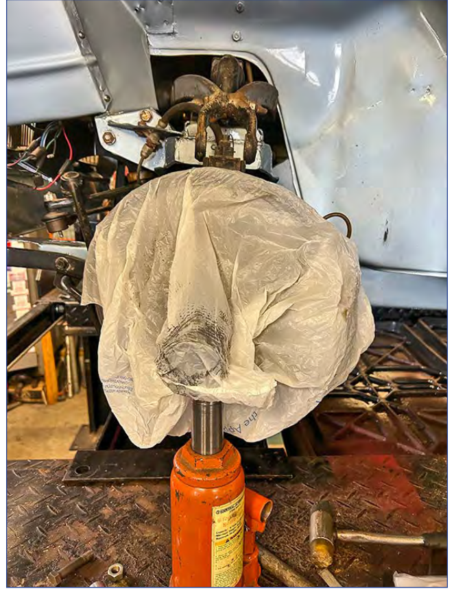
2 Bag over the splined hub protects you from grease marks!
