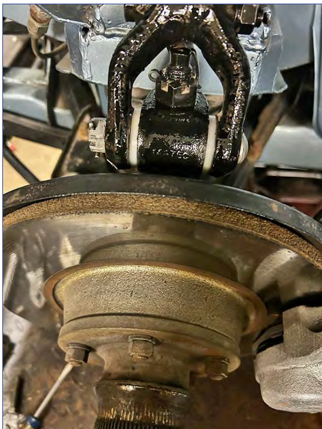
7 New camber adjusting bushings installed!
