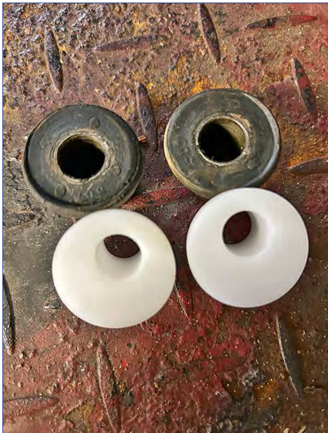
5 Old concentric rubber bushings compared to new eccentric polymer bushings.
