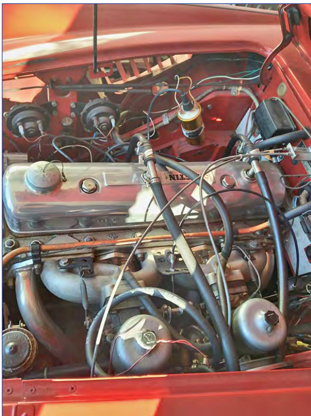
Intake manifold and carb float bowls are not stock.
