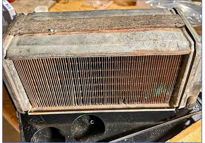
Healey 3000 Heater Core Removed from The Car.
