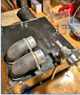
Heater Box, Water Control Valve and Defrost Elbows
