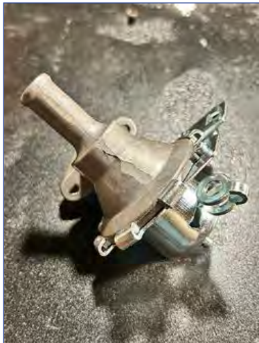
Heater Water Control Valve
