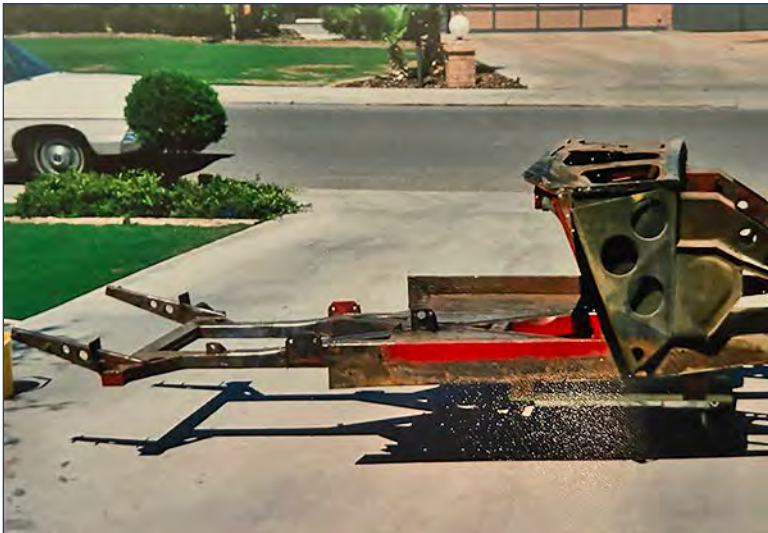
100-6 With Rebuilt Rear-end Chassis.
