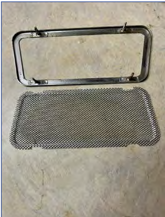
I separated the speaker grille from the surround. It just pops right out.
