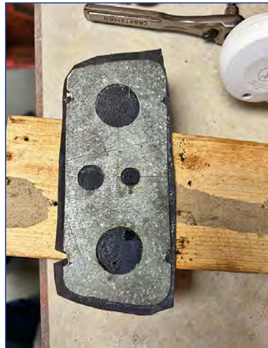
I fabricated a piece of metal with the holes for the different electrical components to fit the speaker grille surround and covered it in vinyl to match the dash.
