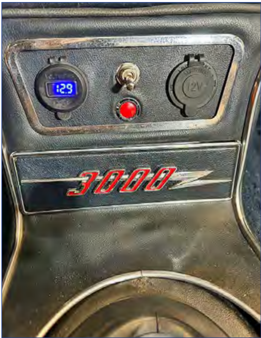
The voltmeter switches on with a push button underneath the rubber cover.
