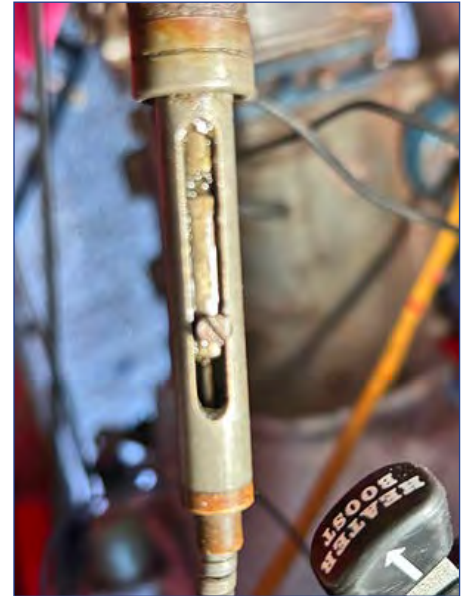
Close-up of Pull Knob Shaft. Note the setscrew (difficult to see) that clamps onto the inner wire of the slide cable.
