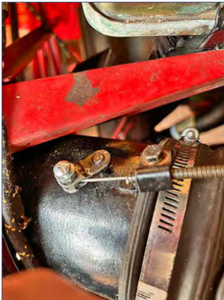
4-Inch Inlet Housing on Left-side of Car Showing Slide Cable Connected to Damper.
