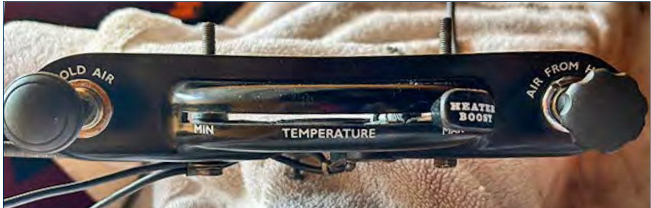
Under-dash Temperature Control Panel Showing Left and Right Pull Switches and Slide Lever in Center. (Not seen are the 3 slide cables that connect to back of panel.)
