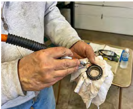
After cleaning the bearings in mineral spirits, we blew out the liquid and grease with an air gun.
