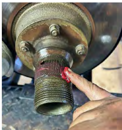
Grease the splines, shoulder and threads.
