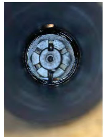
Castellated hub nut with cotter pin access hole lined up at the top.
