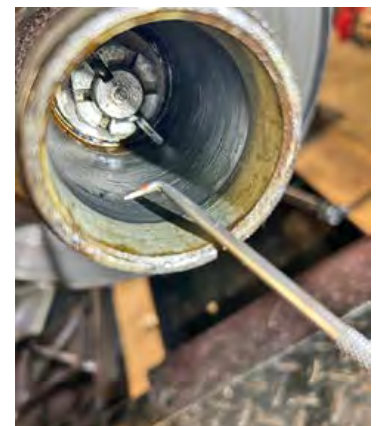
This pick tool works well for pulling the rear leg of the cotter pin or pulling it through the top hole.
