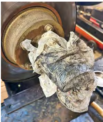
Cover the greasy splines (a plastic grocery bag works well) or you will get grease stripes on your shirt.
