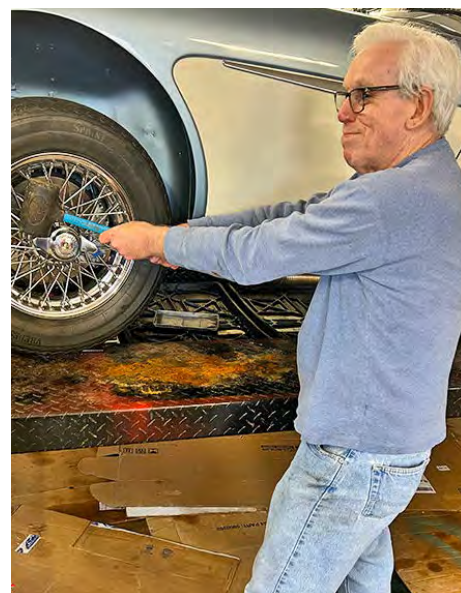
Steve gives the knock-off a few solid whacks to finish the job. We have all done this - you hit the wrong side of the knock-off before figuring out you are actually loosening it, then switch to the correct side!
