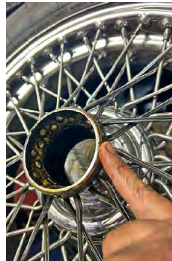
Grease the shoulder on the wheel also!
