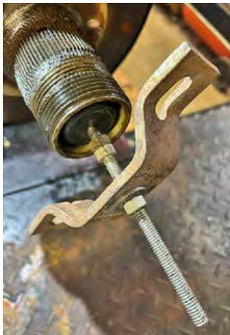
This is my homemade tool for removing the grease cup.
