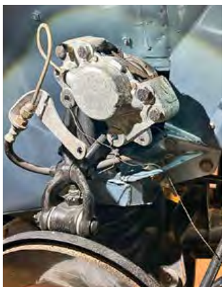
Caliper moved out of the way and wired into place on top of the shock.
