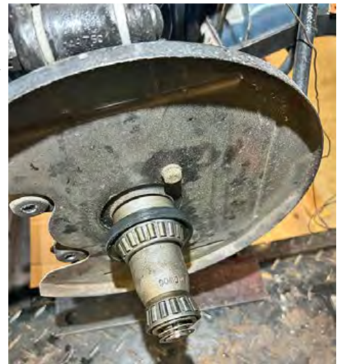
Here are the parts in order - spacer, seal, inner bearing, distance piece, outer bearing, spacers. The tab washer and castellated nut go on the outside.
