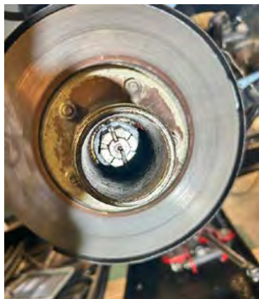
Drop the cotter pin through the access hole into the castellated nut and bend the legs.
