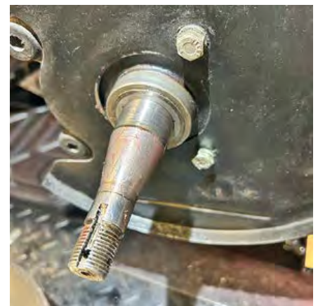
The spacer goes on first, the grease seal rides on this surface. Make sure you grease the outside of the spacer and the inside of the seal.
