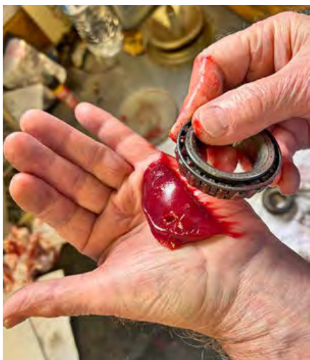
Push the bearing into the grease until it comes out the top. Small side down works best.
