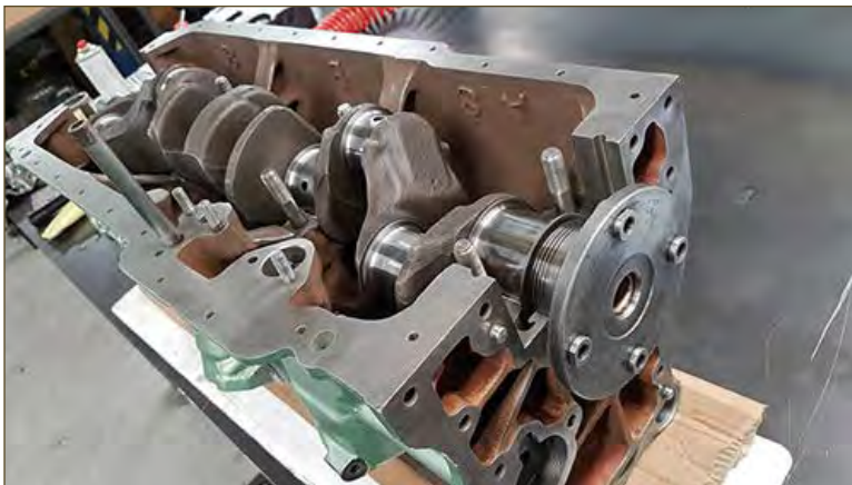
The Archimedes Screw is visible behind the plate that the flywheel mounts to.
